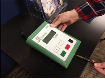
Plug the **power cords** into the wall outlet, power supply, and back of the machine. Plug the **array** into the front of the machine.
